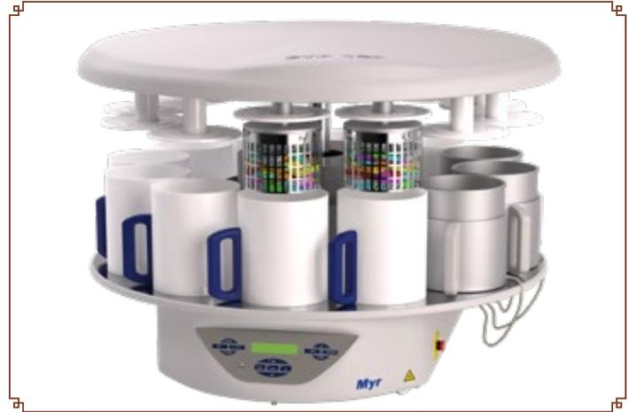
up-and-down movement of the basket (*shaking*). Finally, the basket is placed over the reagent level and starts whirling at 120 rpm in order to minimize reagent carry-over.
