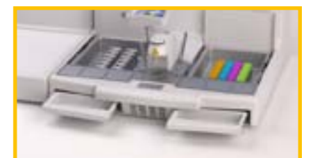
Removable trays for storage of cassettes and molds. Surplus paraffin is drained into waste, removable drawers.
