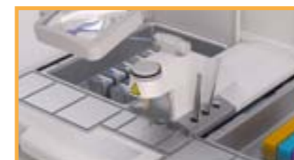
Dispensing area with touch plate or footswitch, light and forceps support
